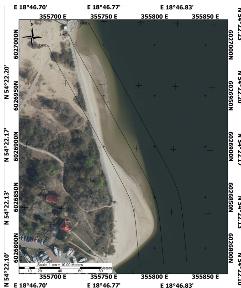
Figure 3. Flight trajectory of the UAV using the LiDAR system in the study area.
