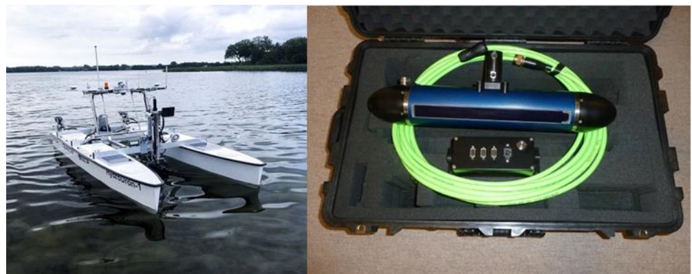
Figure 3. Unmanned vessel HydroDron-1 (left side) and interferometric sonar PING3DSS-DX-450 (right side).
