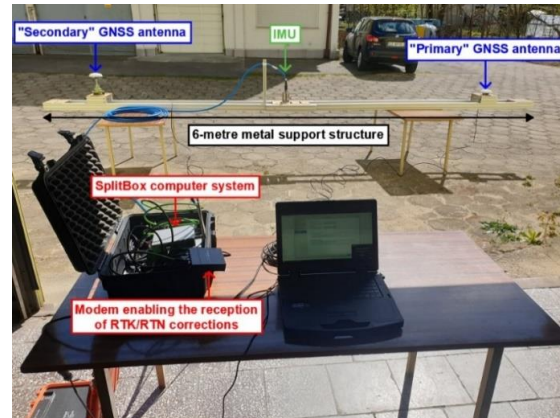
Figure 2. The arrangement of the GNSS/INS system on the metal support structure.
