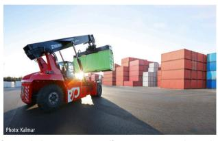
ing to the manufacturer, the battery capacity is sufficient to cover a complete working shift. The charging will be performed during scheduled breaks using combined charging system (CCS) chargers with a maximum capacity of 350 kW, making it the world's first reachstacker to implement this standard. The purchase comes together with five-year-long Kalmar Complete Care that will provide Westport with preventive and corrective maintenance services.
