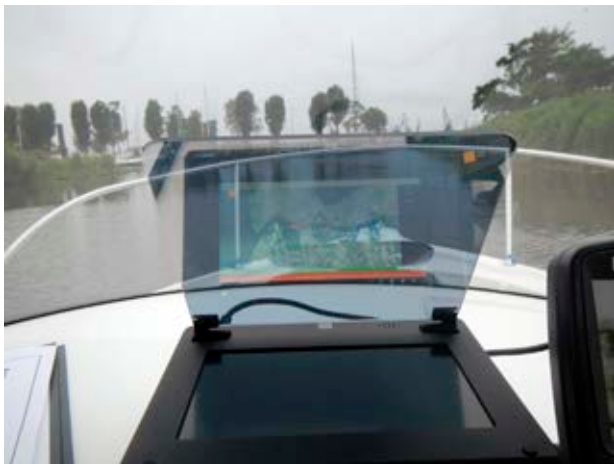
Figure 7. View of tested HUD during real-environment tests on a boat
