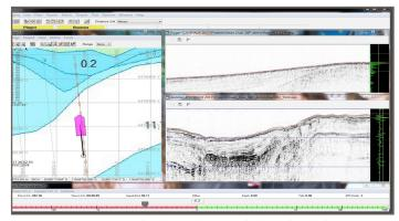
HYPACK® supports both analog and digital sub-bottom systems. It saves your data to industry standard SEG-Y. It's a standard feature in HYPACK®.
