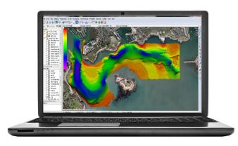
creating sidescan mosaic and create electronic charts (ENC) are part of the package. Over two hundred sensor inputs provide the connection for all types of GPS, Inertial systems, echo sounders, sidescan and sub bottom, magnatometers, velocity sensors and more. HYPACK<sup>®</sup> is more than a navigation software; it's your complete hydrographic package from planning to deliverable.
