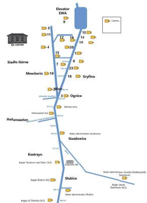
Fig.1. Schema of existing and planned cameras on Odra RIS area. [own elaboration based on 5]
